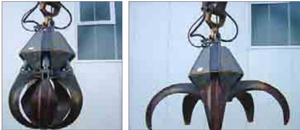
5-tine clamps of a material handler
