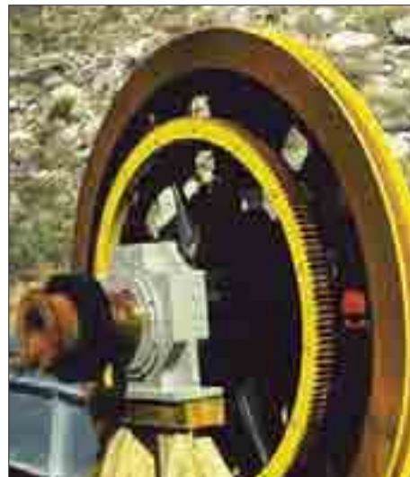
Wheel that winds the metal rope.
